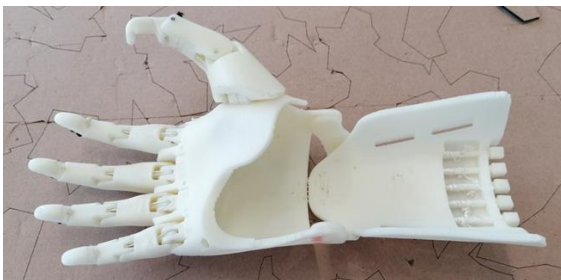
Hand-prosthesis made by Additive Manufacturing (FFF)
